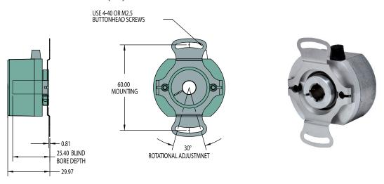
All dimensions are in mm with a tolerance of  $\pm 0.127$ mm or  $\pm 0.254$ mm unless otherwise specified
