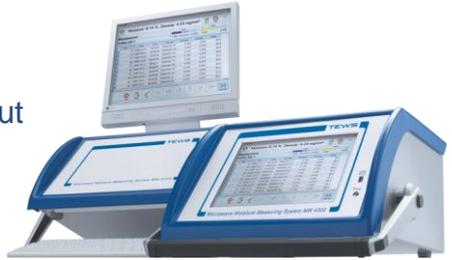
Measurement results are obtained within seconds. As soon as the sample is filled into the sensor, the result will be displayed. Results are stored in the instrument together with the date, time and other operational details. The measurement system or an external PC, can be used to prepare a statistical analysis of results or display a time vs. value chart of sensor readings.
