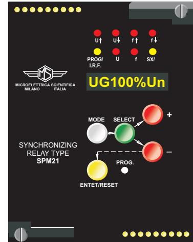
The SPM21 numerical synchronising relay measures voltage and frequency of two inputs; the voltage, frequency and phase angle of the Generator input (G) are individually compared with those of the Bus input (B) considered as reference. The relay includes the following programmable functions:
