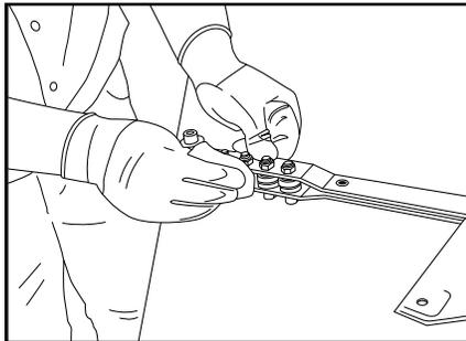
Clean Belt Support Bearings when dirty. Wipe Bearings with a clean cloth and a solvent such as mineral spirits.
