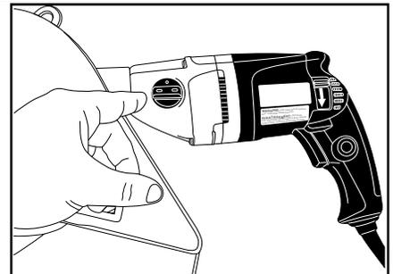
For normal use, operate in Reverse Direction; press drilling direction button for reverse direction operation.
