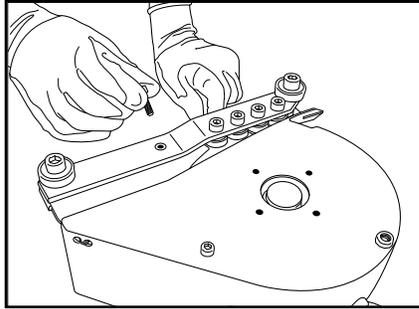
2. Remove Carriage Support Bolt and Nut.
