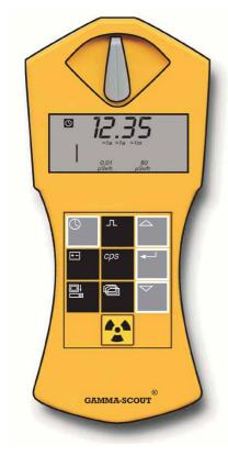
GAMMA-SCOUT® is powered by a 2.7 - 3.7 V lithium thionyl chloride cell. The device will continue functioning until the cell voltage is down to 2.8. When the voltage drops below this value, the battery symbol will appear in the display. The data will be retained, even following a total loss of voltage. The RECHARGEABLE model has a rechargeable battery, which can be recharged via USB (or the power supply unit included with delivery).
