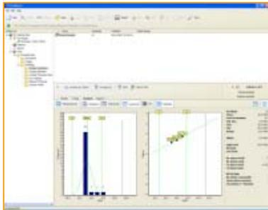
The software has been designed to be familiar and intuitive to any PC user. When the gauge is connected to the PC, individual readings can be sent directly into the software for real time analysis or simply 'drag and drop' a batch from the gauge to the software.
